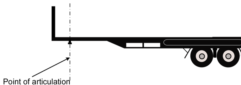
Point of articulation - kingpin for fifth wheel
